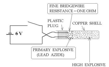
So here's a usual dynamite blasting detonator, about a quarter inch in diameter. A 6-volt signal makes a tiny bridge wire glow red hot, and that starts a primary explosive <u>burning</u>, and that burning rapidly accelerates into a detonation, which starts the high explosive at the end.
