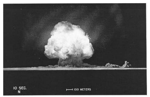
Then the hot gas bubble starts rising. It contains almost all of the original materials of the bomb, the intensely radioactive fission fragment atoms, and the steel atoms of the tower. This will form the mushroom head of the rising column.
