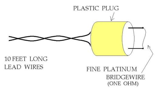
So soon I was holding the wires, with a free plug on the end of them, and I saw that there was a fine bridgewire soldered to the stubby wires projecting through the plug. And I still had all my fingers, and both eyes. (I could easily have been wearing safety glasses!)
