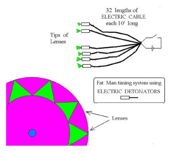
When Alvarez heard of this problem with the primacord timing, he suggested to Kistiakowsky that instead of 32 lengths of primacord, they should use 32 lengths of electric cable, each ending in an electric detonator. The speed of electric signals is 30,000 times faster than the speed in primacord. (There's a 6-volt battery to set them all off)\_But Kistiakowsky smiled and told him that the problem is that electric detonators have a long time delay of milliseconds before the full explosion starts.
