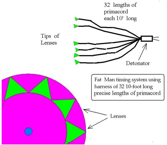
This system of timing the lenses resulted in a scatter of lens timing events in the tens of microseconds, which was not nearly good enough for the requirement, that all the lenses should initiate within a tenth of a microsecond. This scatter was due to slight variations in the propagation speed of the wave in the primacord, and perhaps even the bending pattern of each cord. What was their solution? To try to get DuPont to make better primacord!
