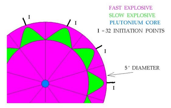
So when 32 of these explosive lens sectors were assembled around the inner sphere, they could produce wavelets that would join up to make the required large converging wave.
