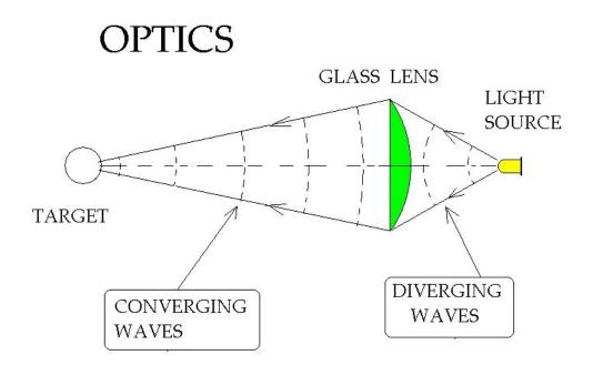
Light travels more slowly in glass than in air, so the central parts of the wavefront get delayed more than the edges. This transforms an outward-going diverging wave into a converging one.
