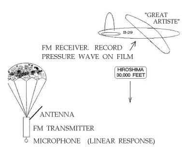
The pressure wave will be received by this special microphone, hanging from a parachute in open air. It will telemeter the data by an FM radio channel to a receiver in our B29, where the pressure signal will be recorded on movie film. This system will be made in triplicate, i. e. three parachutes and three microphones, in case any of the three channels fails to function.
